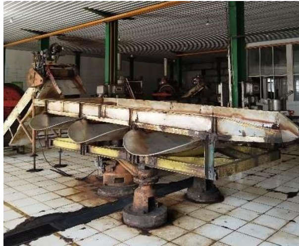
Gambar 7. Alat mesin rotary roll breaker (RRB)
