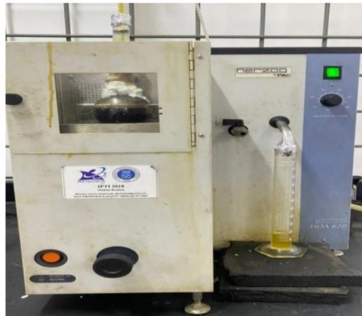
Gambar 2.1 Alat Distilasi ASTM D-86
