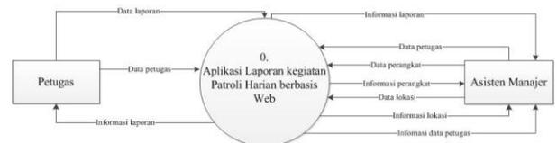
Gambar 5. Rancangan Data Flow Diagram
