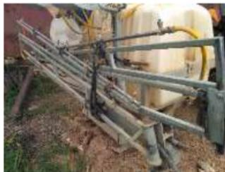
Gambar 41. Rangka *boom sprayer*
