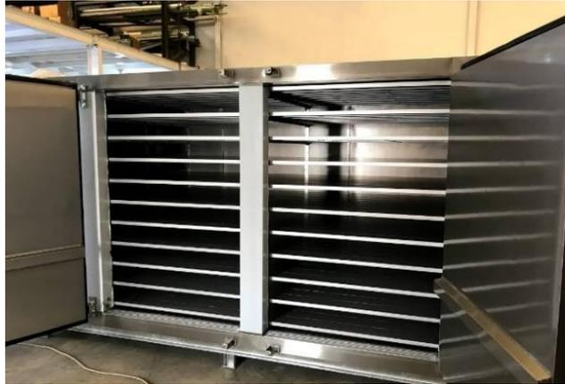
**Gambar 3.** *Contact Plate Freezer (CPF)*
