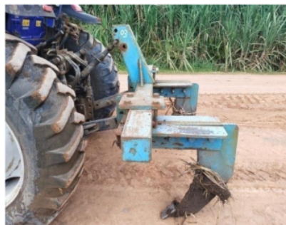
Gambar 5. Implement Subsoiler Parabolic 2 Mata
