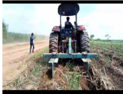
Gambar 3. Implement Subsoiler Parabolic 2 Mata
