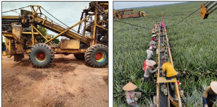
Gambar 7. Alat mesin harvester Cameco type double wings double output
