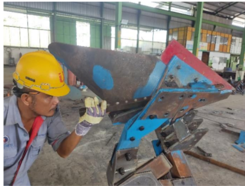
Gambar 13. Proses perakitan implement moldboard plough 3 base
