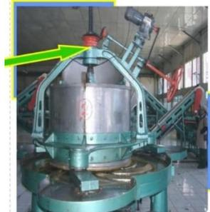
Gambar 3. PCR (*Press cup roller*)
