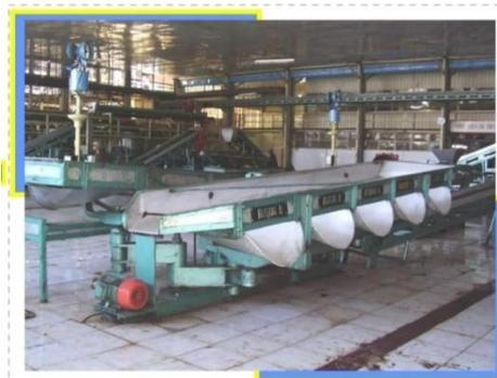
Gambar 4. *Rotary roll breaker*
