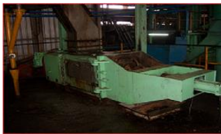
Gambar 3. Screw Press sumber: http://www.fernando413.blogspot.com
