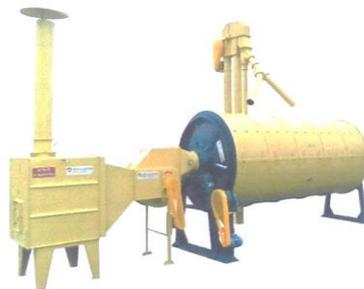
Gambar 5. *Rotary Dryer*
