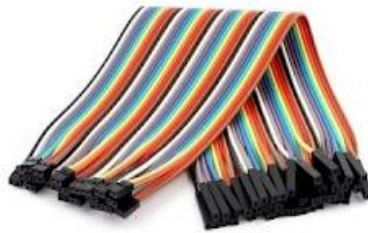
Gambar 12. Kabel Jumper Sumber: (Suryana, 2021)
