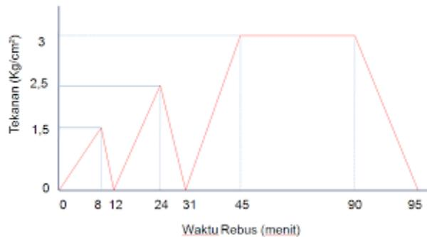
Gambar 3. System perebusan *triple peak*
