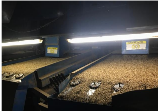
Gambar 10. Mesin De-Stoner Sumber : PT LDC Coffee Indonesia 2021
