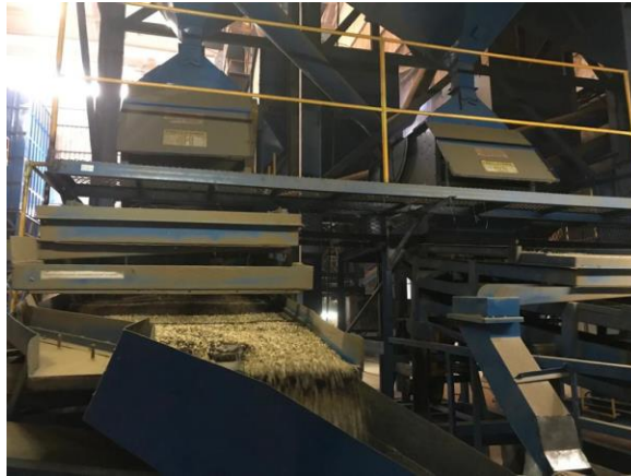
Gambar 7. Mesin Pre-Cleaner Sumber : PT LDC Coffee Indonesia 2021
