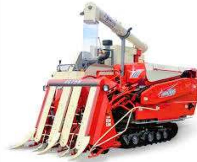
Gambar 2. *Combine Harvester Tipe Head Feeding* (Alibaba.com)
